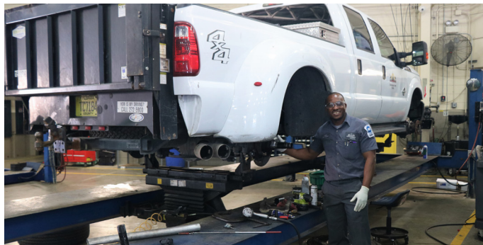
Fleet Technician Frank Okungbowa performing a truck brake change and annual inspection.
