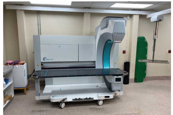
Lodox – Full body scanner allows full body x-ray images to be taken in approx 60 seconds. Used to assist with location of projectiles, foreign objects, injuries, and medical conditions (i.e. enlarged heart).
