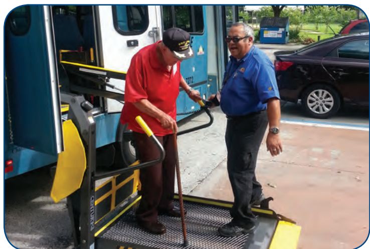
Vehicles are equipped with lifts to assist riders who may have difficulty with steps or stairs or who use wheelchairs or other mobility aides.
