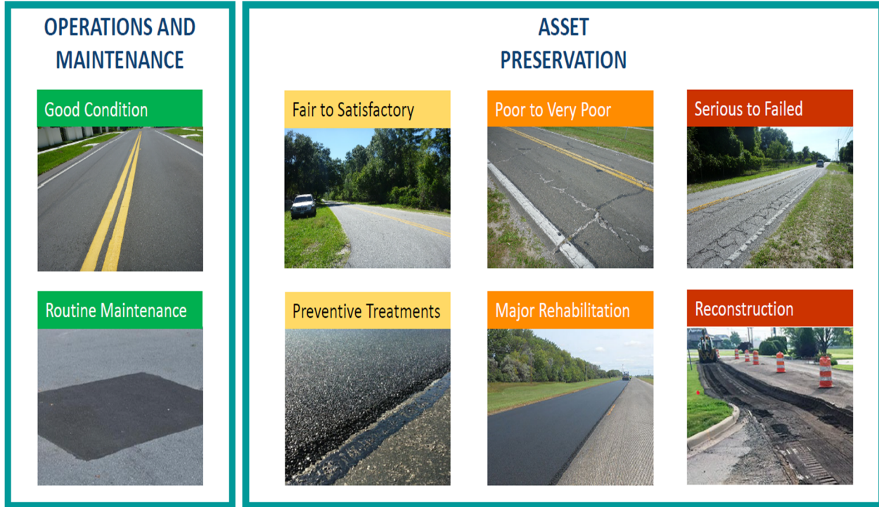
FIGURE 1-3: Road conditions determine the type of work required. Source: Hillsborough County Transportation Workshop Asset Preservation, May 26, 2021.
